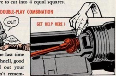
with crud or carbon buildup when you're cleaning your rifle-especially in the bolt and locking recess areaget your armorer to help you tackle it with P-C-111 carbon removing com-Any time you run into real trouble pound, FSN 6850-965-2332, 5-gal pail.
