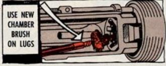
collect under the extractor, the claw won't be able to snap over the rim of a cartridge case. And if gook and brass chips from cases gather in the recesses, your bolt action will be stymied. So, bear down on your bore brush in both these places.
