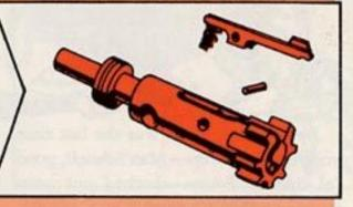
REMEMBER — Watch your lubing. Too much lube speeds carbon buildup in the chamber and bolt locking recess. Same thing with the carrier key. A rag or swab or even a pipe cleaner dampened with LSA will do the trick here. Best bet: Follow the guide on pages 22-24.
