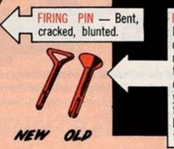
FIRING PIN RETAINING PIN — Bent, busted, badly worn. If one or both tangs are busted, there's no sweat as long as it'll hold the firing pin in place. But, be mighty careful you don't lose it when you're doing PM. A rifle fired with this pin missing may fire once but that's all. The firing pin would then fall out and — no-fire!
