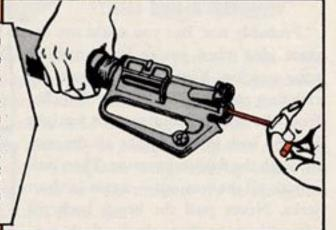
Bolt Carrier: Remove it from your weapon and field-strip it at least once a week. Use bore cleaner with any bore brush mentioned above and attack all parts, especially behind the rings and under the lip of the extractor. Clean the carrier key with your bore brush FSN 1005-903-1296 and bore cleaner. Then dry all the parts real good and coat 'em with LSA.
