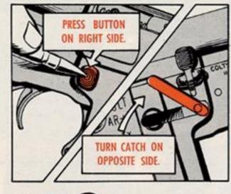
No sweat adjusting the catch the way you want it, either . . . and you're authorized to pull this deal. Just press the button on the right side of the rifle with the nose of a cartridge far enough so's you can turn the catch on the left side of the weapon. You turn the handle clockwise to tighten it and counterclockwise to loosen it. Best of all, you don't have to take the weapon apart to do this.
