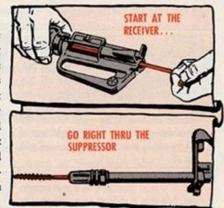
Same idea goes when you're running patches through. Run it all the way through the flash suppressor before you start to pull back . . . no matter what size patches you're using-the one for the M16A1 (FSN 1005-912-4248) or any large type that you have to cut into 4 equal squares.
