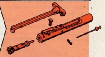
Extractor and Extractor Spring: Double check 'em every day, at least. Eyeball the extractor for chipped or broken edges in the area of the lip that engages the cartridge rim. Replace it if you find it damaged. Test the extractor spring by pressing on the extractor. If the spring's weak, replace it.
