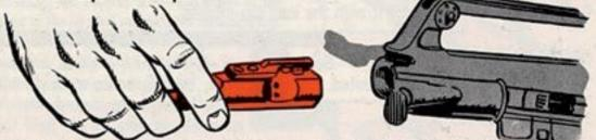
Here's the Pitch: The front end of the gas tube is self-cleaning, thanks to the hot gases and high pressure from the barrel. But, if you don't keep the other end clean — the gas tube area where it mates with the carrier key inside the receiver - brother! You've got to clean this area with elbow grease to prevent stoppages. Hear!
