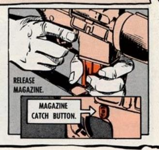
So, take a cue from experience. Adjust the catch button so's it's just about flush with the inner groove or just sticks out a tiny bit. This'll make the catch firm enough to prevent accidentally bumping the button and letting the magazine drop out—yet it won't be so tight that you can't pull the mag out for a quick re-load.
